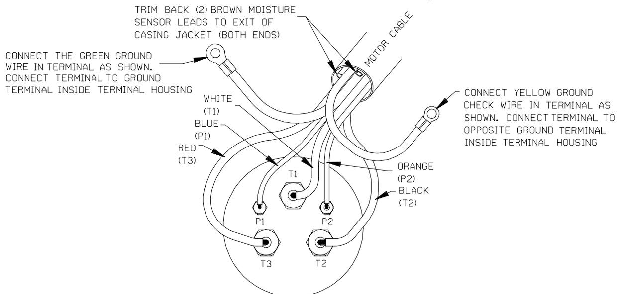
**Figure C-6. Terminal Housing Wiring Connections**
