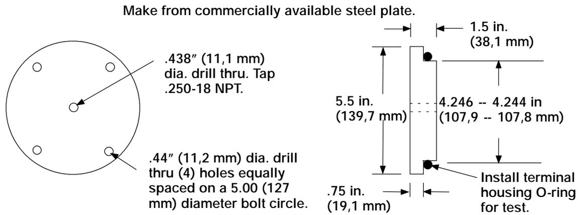
Figure C-9. Motor Vacuum Test Plate
