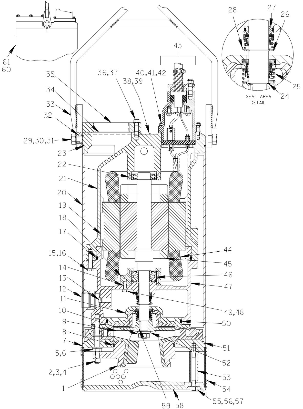
Figure C-1. Typical SM4G And SM4J Series Pump Assembly
