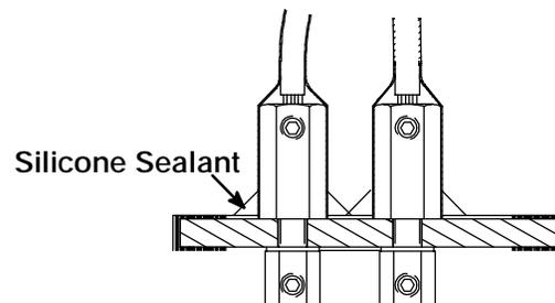
**Figure C-7. Silicone Adhesive Sealing**
