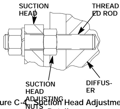
Figure C-4 Suction Head Adjustment Detail
