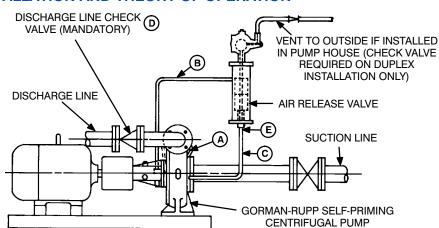
The product recirculates through the return tube assembly "C" to the pump suction. The liquid pressure equalizes the priming pump spring pressure and the priming pump slides into neutral. At this point, the pump is fully primed.
