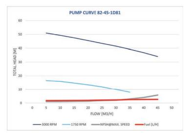
The Gorman-Rupp 82-45-1D81 is designed as a versatile and robust dirty water pump set. At the heart of this compact unit is the Gorman-Rupp 82H52 pump. Designed for a variety of pumping applications, the Gorman-Rupp 80 Series® pumps have been a proven concept for use on construction or industrial sites for many years.
