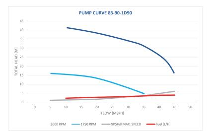
The Gorman-Rupp 83-90-1D90 is designed as a versatile and robust dirty water pump set. At the heart of this compact unit is the Gorman-Rupp 83B52 pump. Designed for a variety of pumping applications, the Gorman-Rupp 80 Series® pumps have been a proven concept for use on construction or industrial sites for many years.
