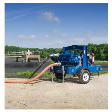
With 4" suction and discharge ports, this selfpriming, positive displacement, hydraulic piston pump can pass up to 2-1/4" diameter solids without damaging or clogging the pump, while maintaining flows of up to 226 GPM.
