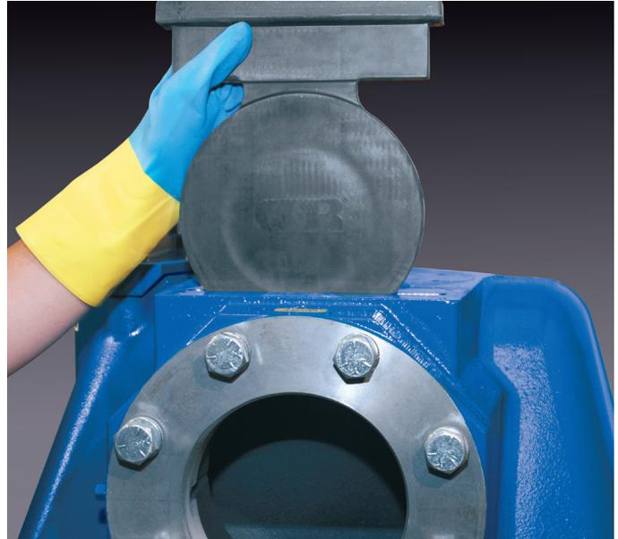
**The suction check valve on Ultra V Series pumps is externally removable eliminating the need to disconnect from piping for inspection or replacement.**
