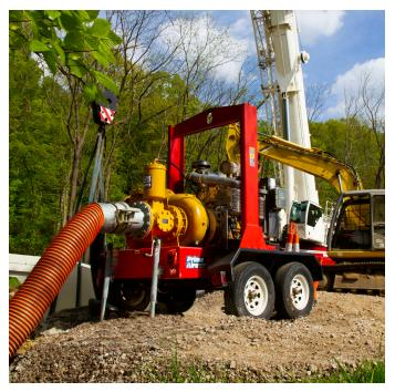
Gorman-Rupp rental pumps are available in sizes from 4" to 12" and depending on the application, suitable for clean liquids or liquids containing large solids.
